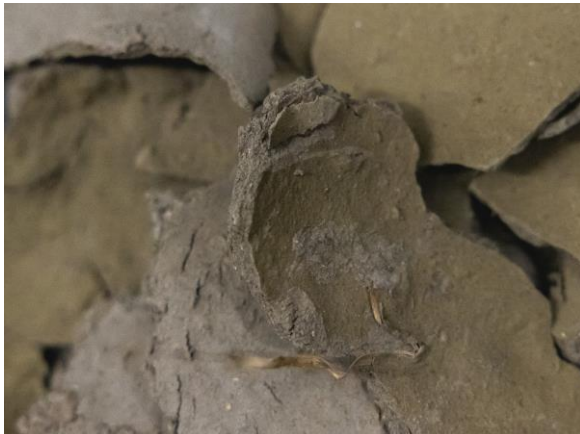
Outgoing Sludge Sediment after the Freeze Dewatering Process with FDWU. Incoming sediment dry solids (TS) content 4-6%.
