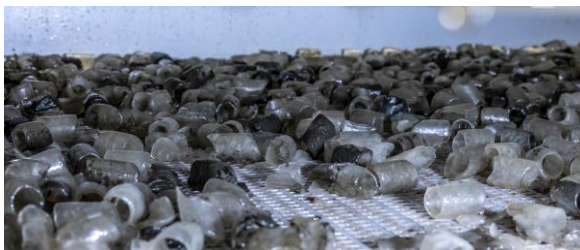
Sediment Sludge in the Thawing/Drying Stage on a THAW COLLECTOR Connected to FDWU
