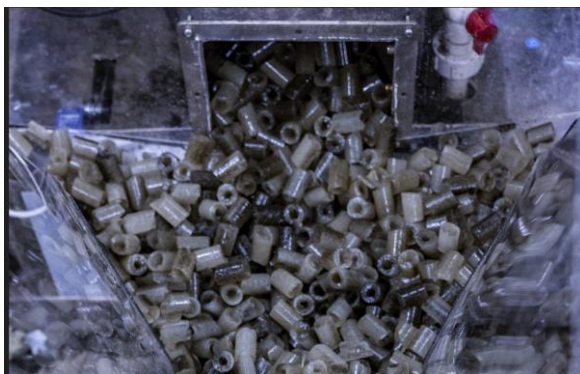
Exiting from the FDWU to an elevator that lifts the frozen sediment up to the THAW COLLECTOR
