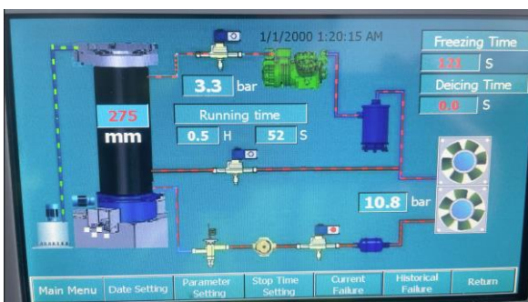
Control System Process Overview for FDWU
